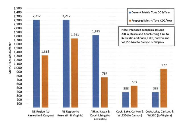
Figure 4-4: NE MN Transportation Analysis: Current vs. Proposed Metric Tons of CO<sub>2</sub>/Year
